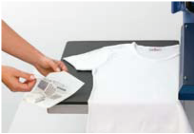
1 Peel off the white protective film*.
