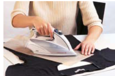
3 A Teflon® underlay protects the soleplate of the iron from any glue residue.
