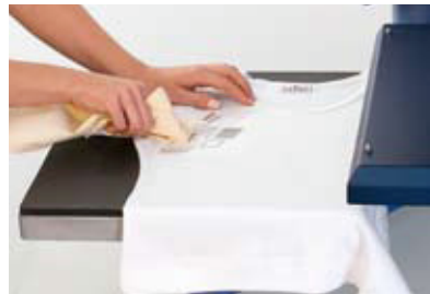
5 After the application is finished, use a pressing cloth to apply additional pressure to the product.
