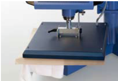
4 After the pressure, time and temperature is set, close the heat press.
