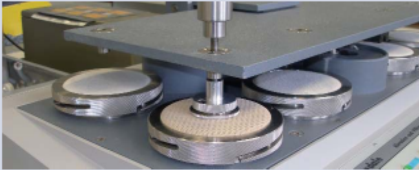
Martindale Test Method for abrasion resistance
