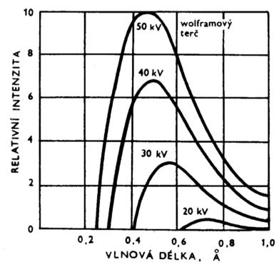
minimum wavelength exists, which depends on acceleration voltage
