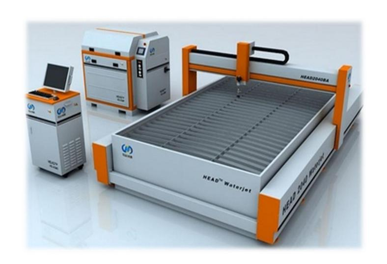
The cutter is commonly connected to a high-pressure water pump (a local water main does not supply sufficient pressure) where the water is then ejected out of the nozzle, cutting through the material by bombarding it with the stream of highspeed water.
