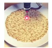
Laser cutting is a technology that uses a laser to cut materials, and is typically used for industrial manufacturing. High-power laser is given to the fabric by computer. Then the material is cut but different type of materials give different type of reacts such as melting, vaporizing, burning etc. This machine works very fast. Maximum speed of this machine is 600 mm/s.
