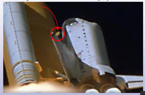
A small piece of insulating foam was released from the tank and hit the left wing of the shuttle during the start.
