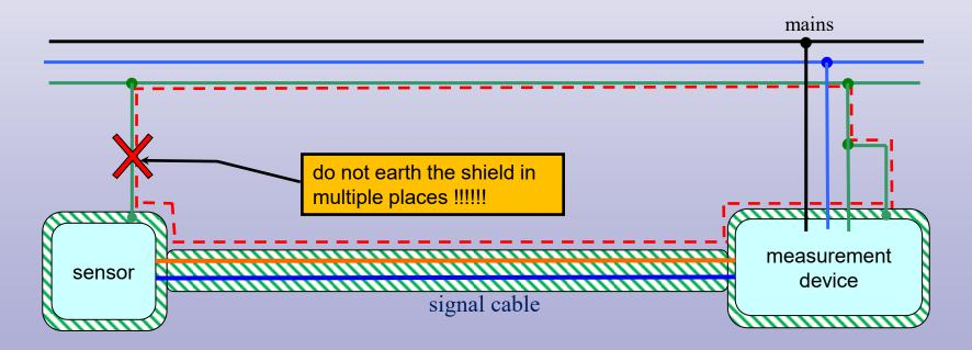
Example of the measurement device correct connection
