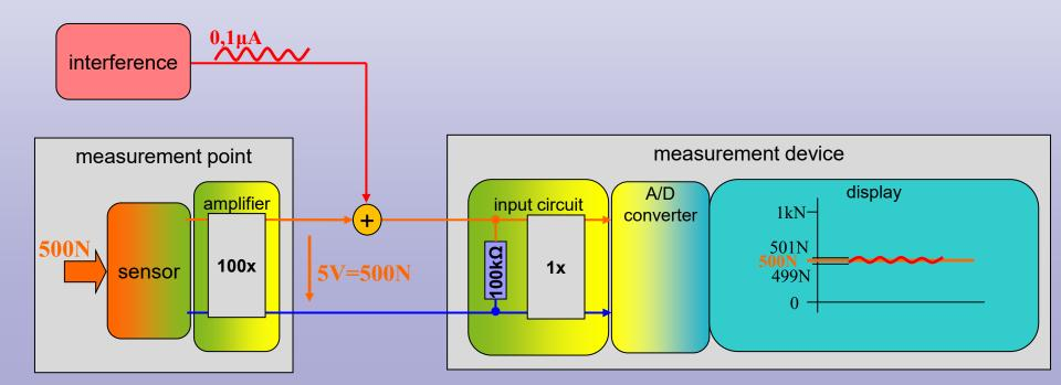
separate sensor and amplifier, industrial version – signal 4-20V:
