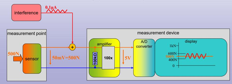
separate sensor and amplifier, laboratory version – signal 0-10V:
