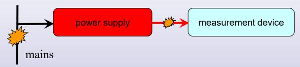
• If the distributed measurement device has multiple power supplies, the earth loop will occur if the power supplies are not connected properly. This is very dangerous, the measured signal can be completely destroyed in this case.
