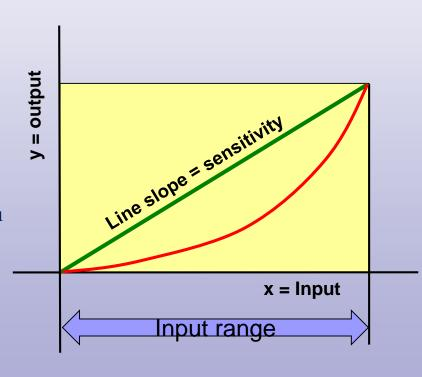
• static conversion characteristic is valid only if the input quantity is within the range !!!!
