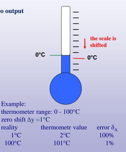
the additive error hyperbolically distorts the output, that is, most at the beginning of the range
