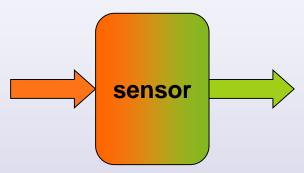
sensor converts the monitored physical quantity into electrical physical quantity (voltage, current, ....)
