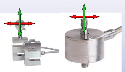
the sensor signal is sensitive to parasitic lateral load - forces or torques
