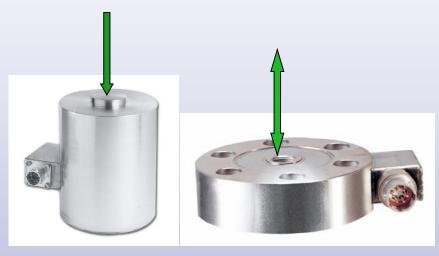
the sensor is insensitive to parasitic lateral load - forces or torques
