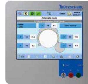
The fields highlighted in blue show the recommended optimisations determined by TCON.
