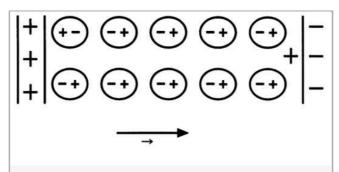
Fig. 6: Generation of free charges in a dielectric through polarisation of the molecules in the electric field of a plate capacitor.
