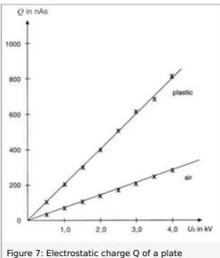
Figure 7: Electrostatic charge Q of a plate capacitor as a function of the applied voltage  $U_c$ , with and without dielectric (plastic) between the plates (d = 0.98 cm)
