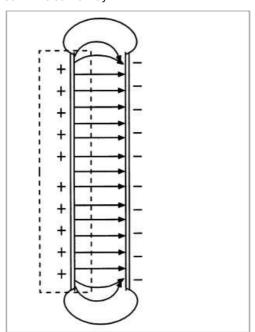
Fig. 3: Electric field of a plate capacitor with small distance between the plates, as compared to the diameter of the plates. The dotted lines indicate the volume of integration.
