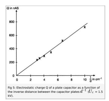
The volume indicated in fig. 3, which only encloses one capacitor plate, was taken as volume of integration. As the surface within the capacitor may be displaced without changing the flux, the capacitor field is homogeneous. Both the flow and the electric field  $\vec{E}$  outside the capacitor are zero, because for arbitrary volumes which enclose both capacitor plates, the total enclosed charge is zero.
