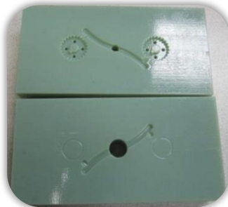
Material injected- Acetal (POM) - 30 parts were injected
