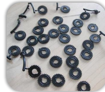
Material injected- Acetal (POM) - 30 parts were injected
