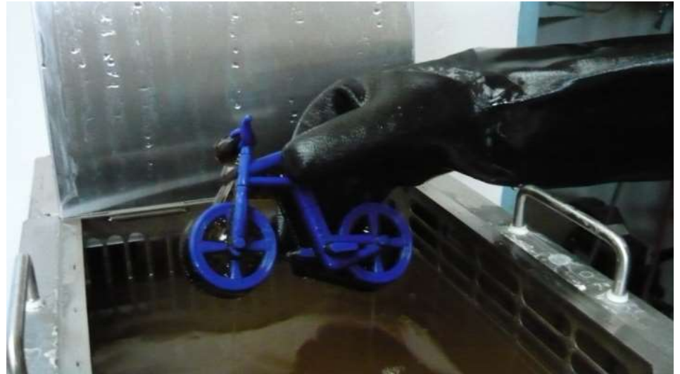
insertion into the liquid (solution with sodium hydroxide) to dissolve the supports
