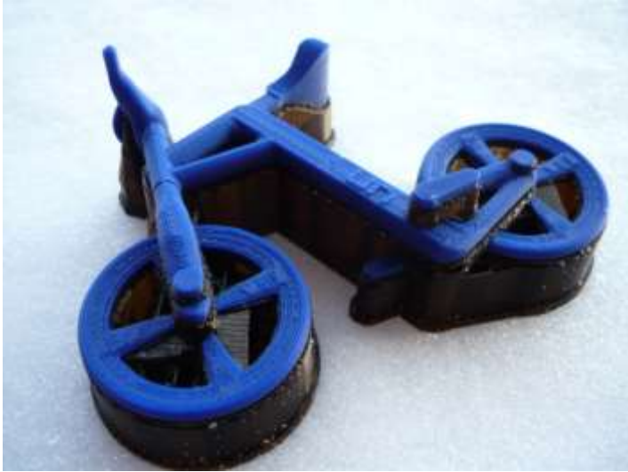
finished part, including supports
