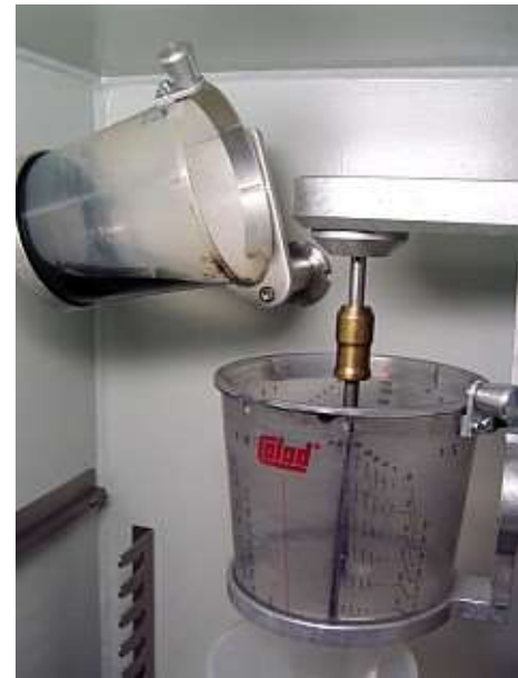
mixing the two resin components in vacuum
