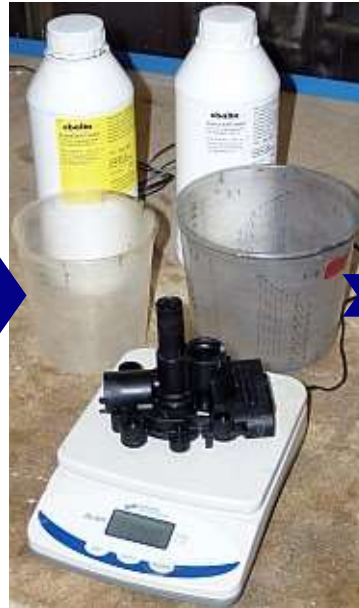
weighing of casting resin components
