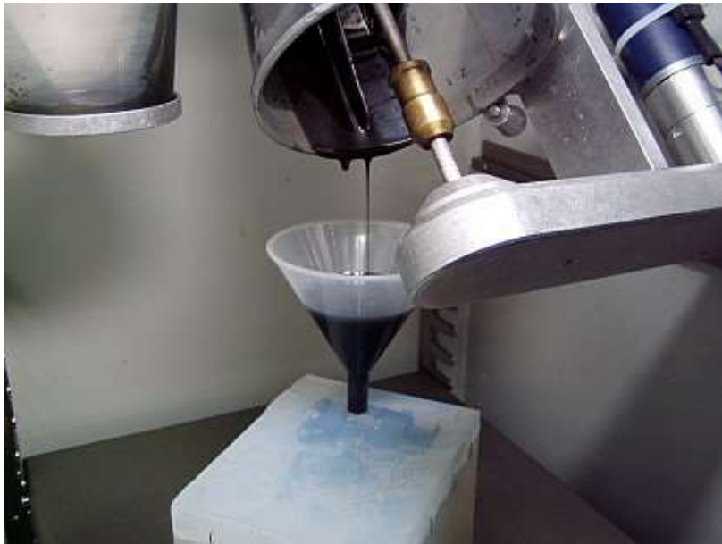
casting resin into the mould
