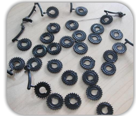
Material injected- Acetal (POM) - 30 parts were injected
