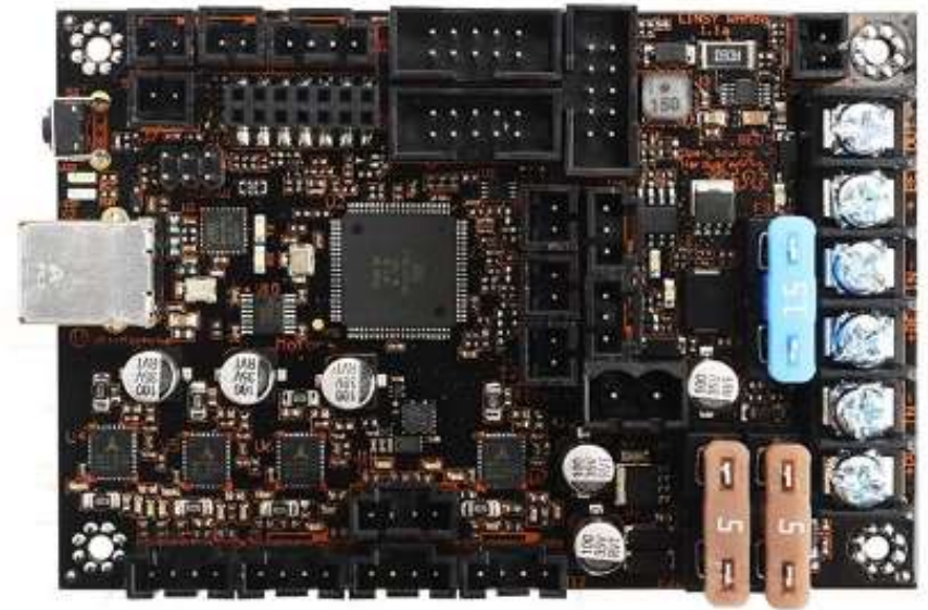
Control board Einsy Rambo 1.1a with integrated drivers for stepper motors (4 x Trinamic TMC2130)
