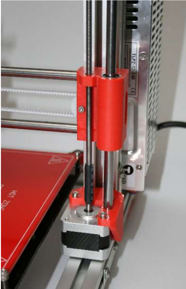
Threaded rod M6 and flexible hose coupling
