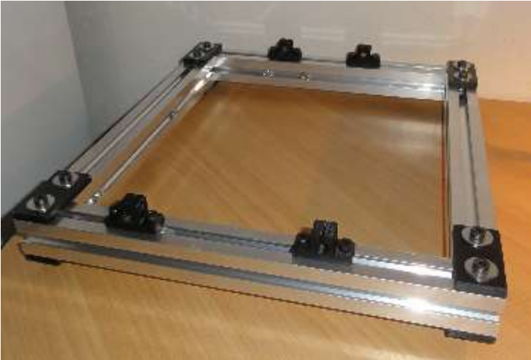
The bottom frame of the Rebel 2 printer, where the "combi" profiles connect the printed plastic plates
