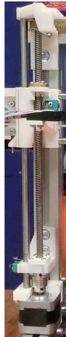
Drive with a trapezoidal screw mounted in bearings at both ends, connected to the motor via a flexible coupling
