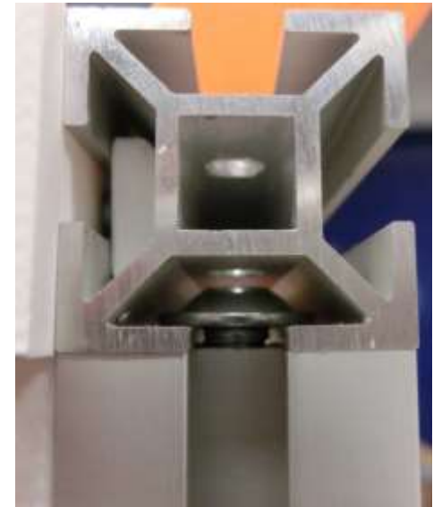
Connection of "combi" profiles via threaded insert and M6 screw
