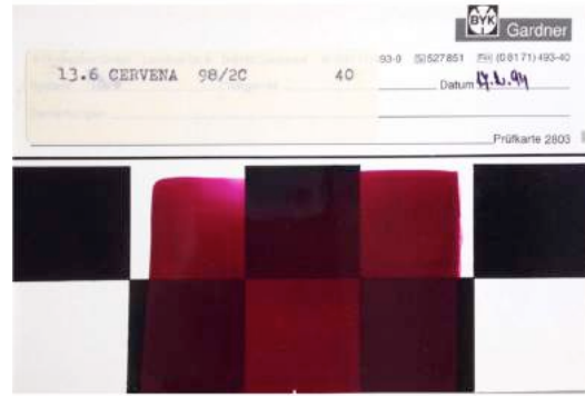
Figure 7.23 Example of hiding power measurement on Gardner contrast paper board – increasing the amount of paint in small increments until reaching the point of essentially complete hiding at which the of visual contrast was considered negligible
