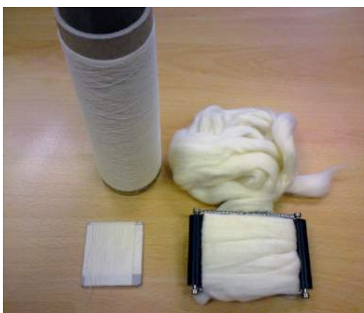
Figure 7.11 Yarn winded on small cavity, Card Wound, free sliver and sliver inside of skein holder
