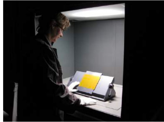
Figure 7.3 Example of correct conditions during visual assessment – office light is turn off, booth is placed in dark room
