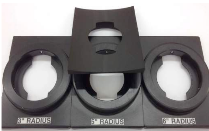
Figure 7.16 Set of accessories (positioning device) for measurement of tubular samples with different diameter (HunterLab)
