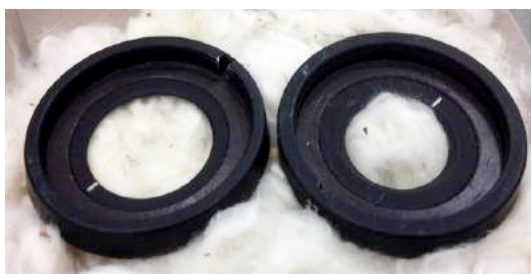
Figure 7.9 Example of sample inherece through measuring aperture without cover glass (right side) and effect of cover glass (left side) on sample
