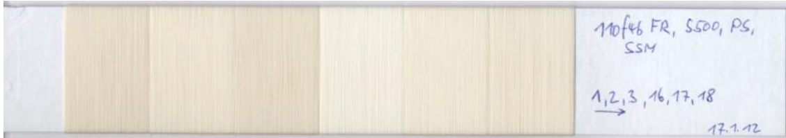
Figure 7.15 Example of individual trials of polypropylene filament wound on Card Wound by parallel method
