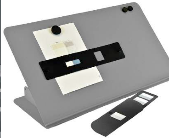
Figure 7.7 Illustration of usage of angle table and rectangle covering mask in case of evaluation of diming in stability tests. Square mask is used for evaluating of color differences, picture is from materials produced by VeriVide, UK
