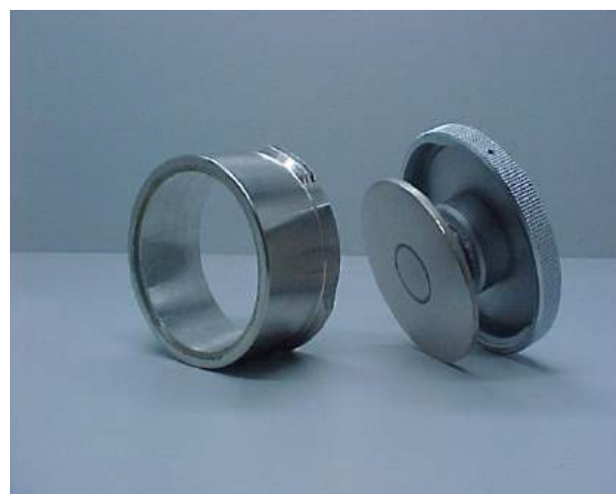
Figure 7.12 Accessory with cover glass for measurement of carved carpets – sample is protected about penetration into measuring device
