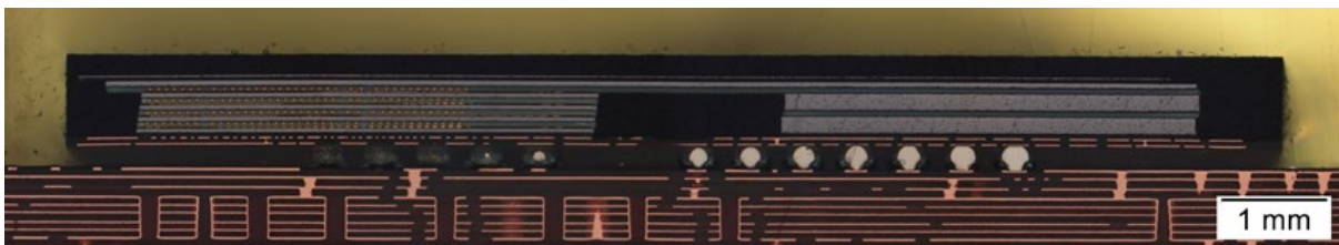
Figure 4.6 Cross-section of a commercial component including various semiconductor chips. Image and preparation: Fraunhofer IZM 41,42
