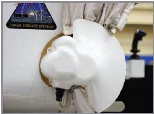
This rover, which has a pressurized cabin to support astronauts, includes about 70 FDM parts, including housings, vents and fixtures.
