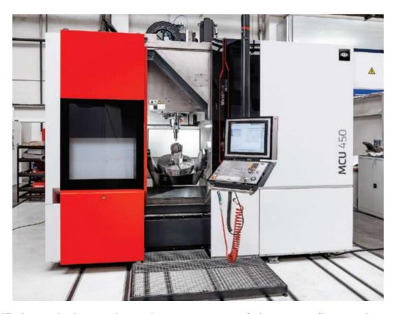
The WeldPrint 2 is based on the concept of the new five-axis milling machine MCU 450 with a portal support structure.
