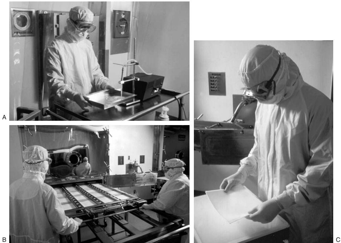
FIG. 10. Manufacturing process of Integra Dermal Regeneration Template. Bovine tendons are cleaned, frozen, processed into a slurry with glycosaminoglycans, and freeze dried into sheets.
