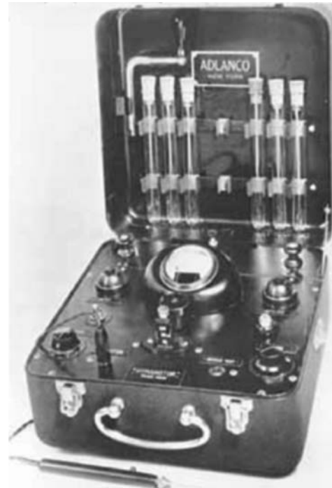
FIG. 7. The Albert Hyman Model II portable pacemaker, circa 1932–1933. (With permission of NASPE Heart Rhythm Society.)
