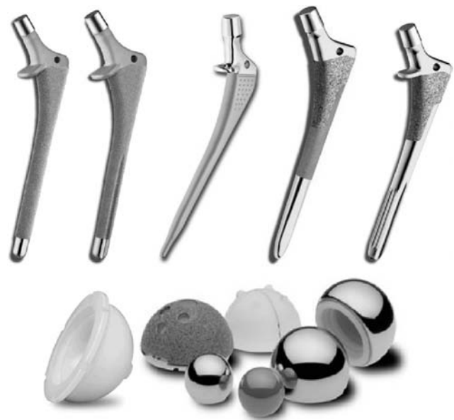
FIG. 3. Examples of a typical current total hip arthroplasty (THA) components available from a single manufacturer, titanium alloy stem, with a cobalt-base alloy (ASTM F-75) modular head bearing on an ultrahigh-molecular-weight polyethylene (UHMWPE) liner within a titanium alloy cup. Also shown is a ceramic head and three acetabular sockets with various surfaces for both cemented and cementless fixation. From left to right the stems are all components of the Versys Hip System (Zimmer Inc., Warsaw, IN) and from left to right are designated Beaded Fullcoat, Beaded Fullcoat with distal flutes, Cemented, Fiber Metal Taper, and Fiber Metal Midcoat. (Photographs courtesy of Zimmer Inc.)
