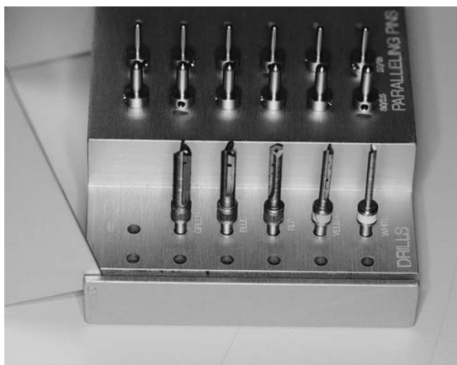
FIG. 16. A variety of instruments is used to create precise holes within the bone for the root-form implants. Twist drills, bi- and tri-spade drills (two cutting edges and three cutting edges, respectively), as well as bone taps to thread the bone all help to make an exacting atraumatic procedure. This set of color-coded drills designed by Cranin and produced by the Brasseler Corp. is available in its own sterilizable carrier. Each drill is no more than 500 \mu\text{m} greater in diameter than the next in the series. These small increments ensure greater and less traumatic drilling accuracy. The final osteotomies are threaded with the specific bone taps made by the company that supplies the root form implants. They are used at speeds as low as 6 rpm and have hollow cores that allow passage of a bone-cooling irrigant.
