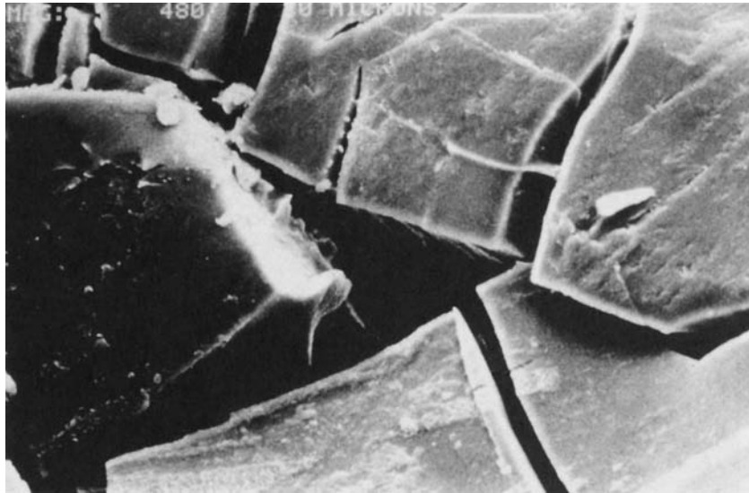
FIG. 16. Random crack pattern of Pellethane 2363-80A lead insulation caused by metal ion-induced oxidation. \times 480 .
