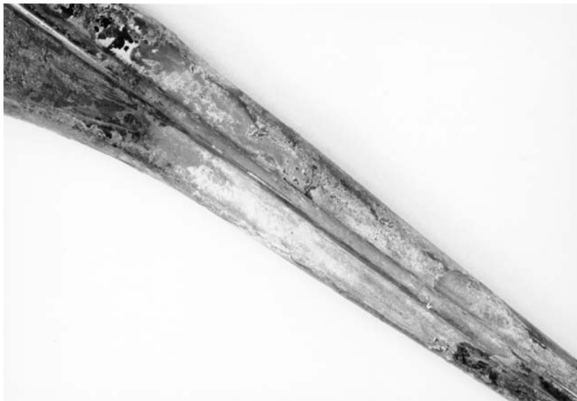
FIG. 5. Extensive corrosion on the titanium stem of a modular hip prosthesis.
