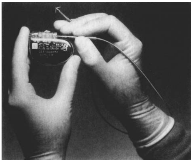
FIG. 10. Cardiac pacemaker with polyurethane lead, tine, and connector. Courtesy of Medtronic, Inc.
