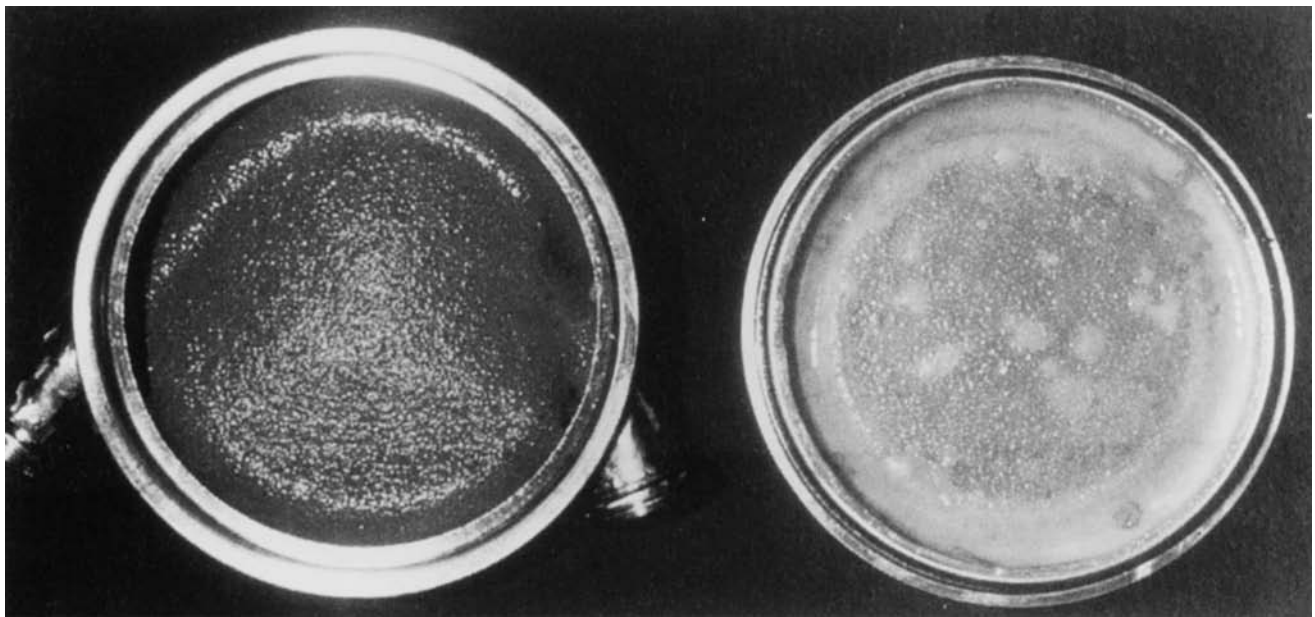
FIG. 5. Pseudointima developed on the interior textured surfaces of the HeartMate VAD after an implantation period of 243 days. On the left is the titanium surface with sintered microspheres and on the right is the textured polyurethane surface. (Reprinted from V. L. Poirier, Thorac. Cardiovasc. Surg. 47(suppl): 316–320, 1999.)
