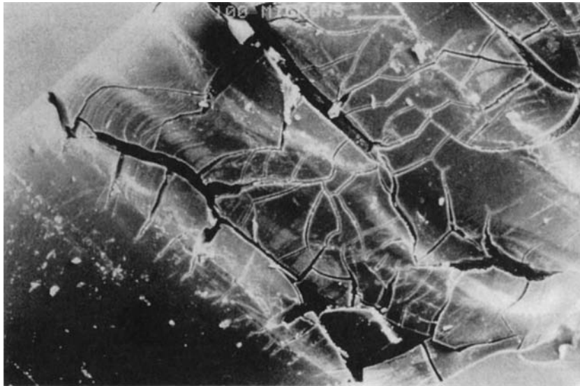
FIG. 18. Crack pattern on inner lumen of polyether urethane lead insulation tracking coil indicative of metal ion-induced oxidation. \times 100 .
