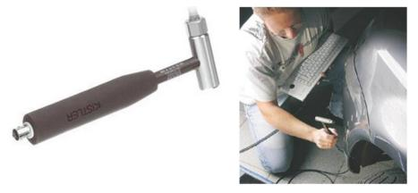
If a hammer with a sensor is not available, a normal hammer can be used, and the measuring can be repeated several times. If the measured results are identical, the excitation is OK.
