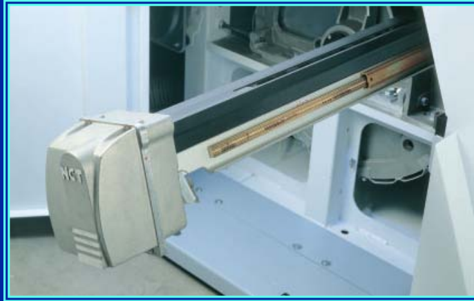
The nep sensor is mounted to the card on a telescopic rail without any problems
