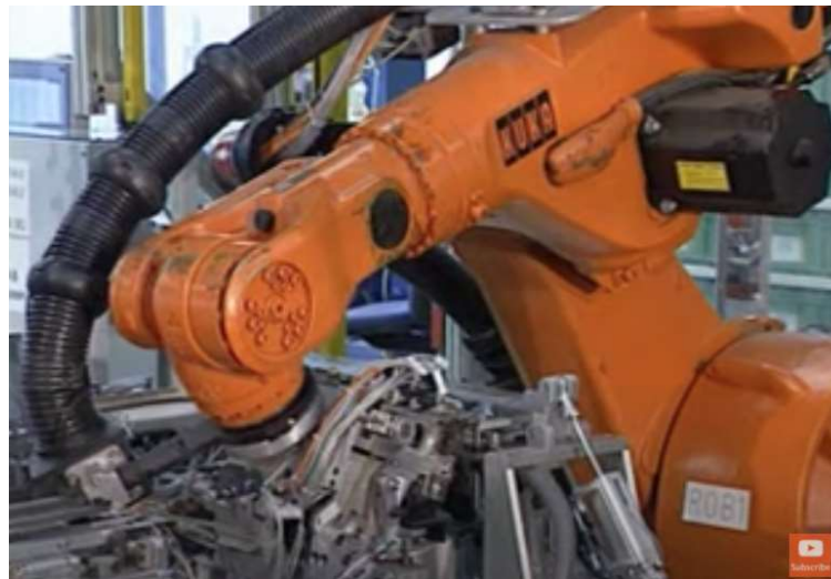
KUKA robot sews car seat covers
