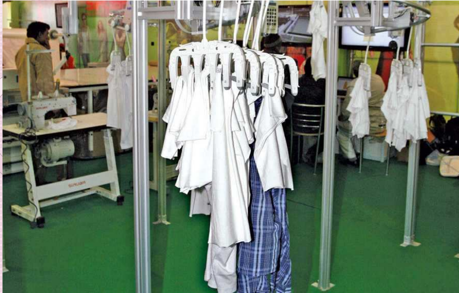
Evans, S. Overhead material handling system in sewing floor [online]. ©2021. Available from: https://www.clothesoneday.com/overhead-material-handling-system-in-sewing-floor
