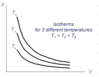
When the air is gradually compressed, the product of pressure and volume is the same in all cases. The volume decreases, and the pressure increases.
