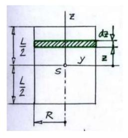
According to the scheme, the volume of the elemental mass:
