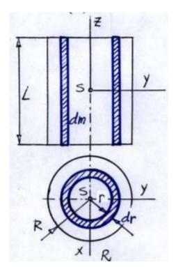
According to the scheme, the volume of the elemental mass:
