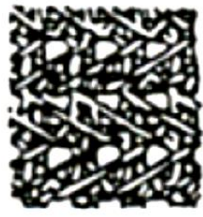
Warp knit laid in warp
