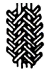
Tubular braid laid in warp
