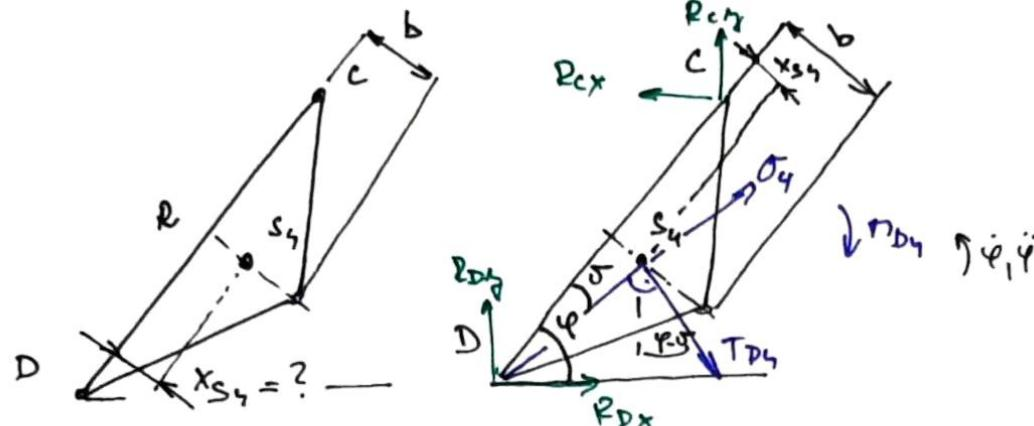
$$\begin{aligned} \text{1. Jelenet je 2. dátum!} \\ (4) \quad & \vec{x}: -R_{Cx} + R_{Dx} + O_4 \cdot \cos(\varphi - \delta) + T_{Dy} \cdot \sin(\varphi - \delta) = 0 \\ & \text{2. Jelenet je 2. dátum!} \\ & \vec{y}: R_{Cy} + R_{Dy} + O_4 \cdot \sin(\varphi - \delta) - T_{Dy} \cdot \cos(\varphi - \delta) = 0 \\ & \vec{z}: -R_{Cx} \cdot R \cdot \sin \varphi - R_{Cz} \cdot R \cdot \cos \varphi + T_{Dy} \cdot \sqrt{\frac{b^2}{4} + x_{S4}^2} + M_{Dy} = 0 \end{aligned}$$
