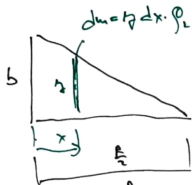
$$J_{S2} = \int_0^{\frac{R}{2}} x^2 \frac{2b(\frac{R}{2}-x)}{R} \rho_2 dx - \int_0^b x s_2 dx - \int_0^{\frac{R}{2}} \frac{2b}{R} x^3 dx = \frac{1}{24} b R^3 \rho_2 - \frac{1}{32} b \rho_2 R^2 + \frac{1}{96} \rho_2 b R^2$$
