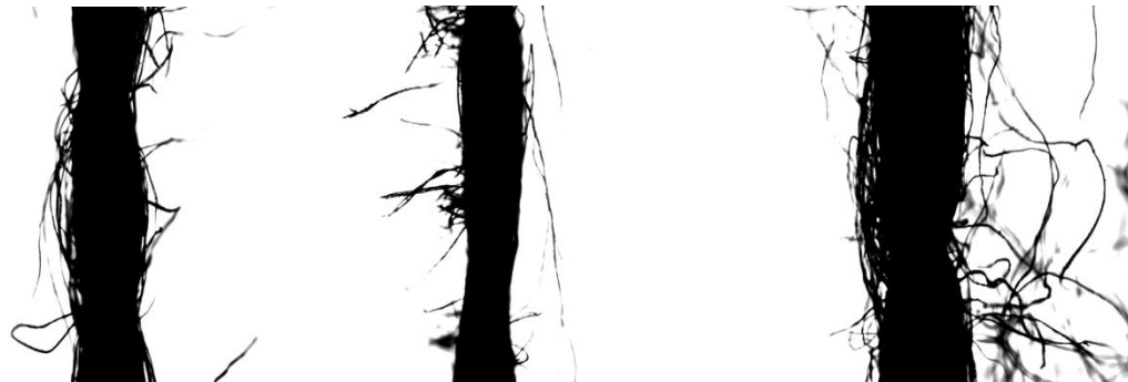
Fig. 2a, b, c: 100% CO 2x29.5tex before post-stress abrasion 50% of the cycles required to damage the yarn (calibration 3.67mmpx-1, image resolution 548px x 704px)
