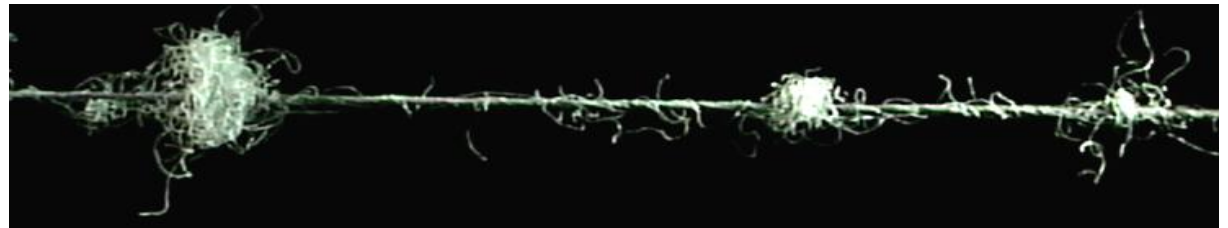
Fig. 1: 100% CO 2x29,5tex - after abrasion stress 50% of the cycles required to damage the yarn (calibration 3,72mmpx-1, image resolution 548pxl x 704pxl)
