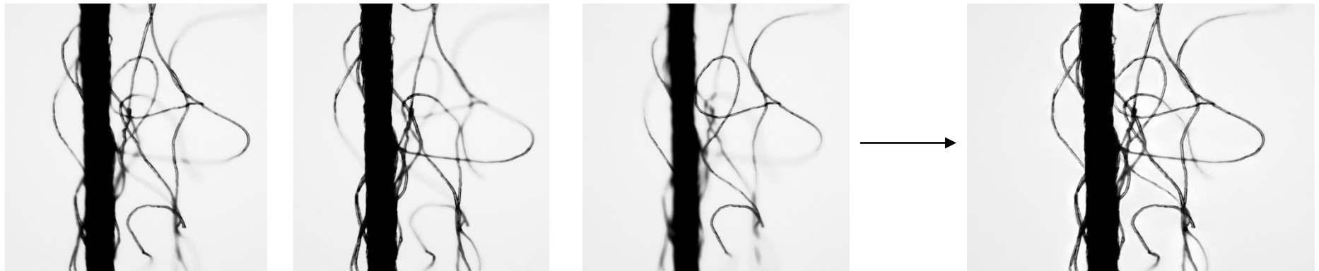
FINAL IMAGE THROUGH THE FUNCTION OF EDF – extended depth focus
