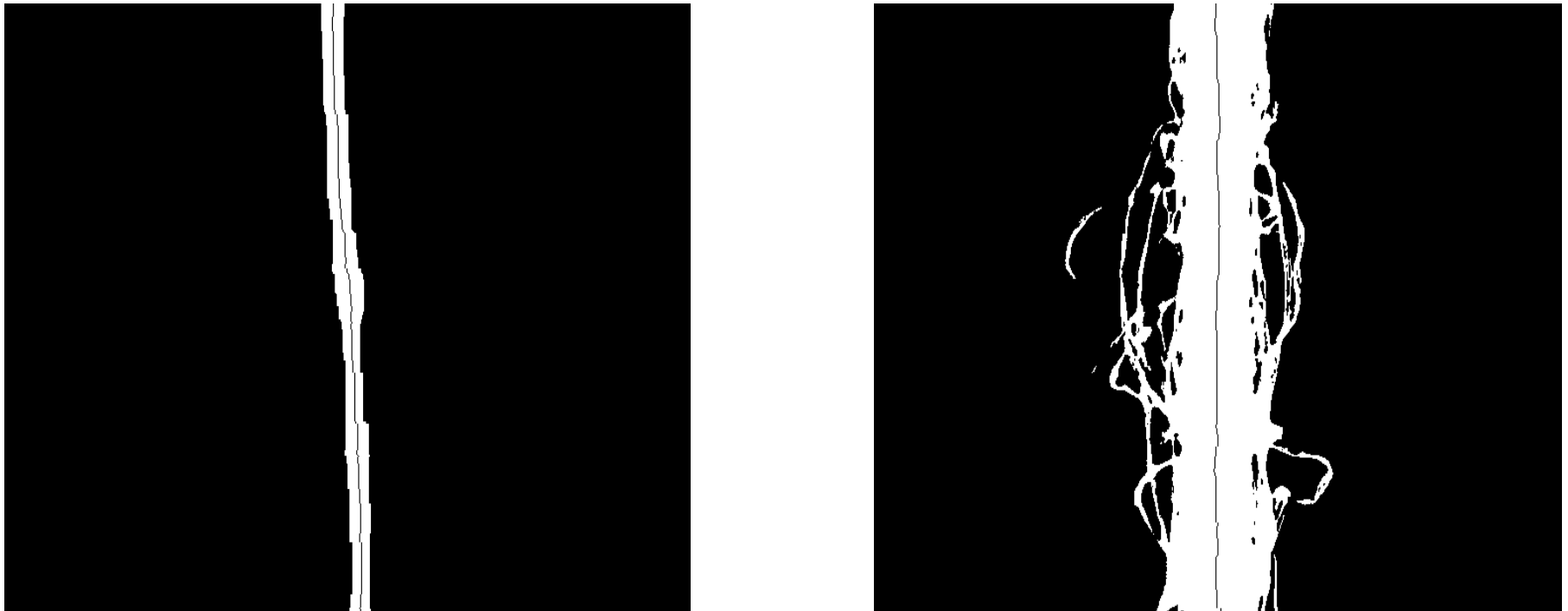
Fig. 17a, b partial processing of images – binary images (open end yarn 72 tex am 85 ktex 2/3 m -1 )
