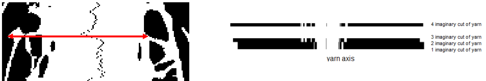
Fig. 20 An example of creating a sum matrix for hairiness curve - the influence of method used for yarn axis determination
