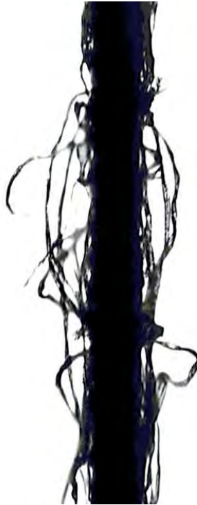
Fig. 16 longitudinal view of yarn – colour image (open end yarn 72 tex am 85 ktex 2/3 m -1 )
