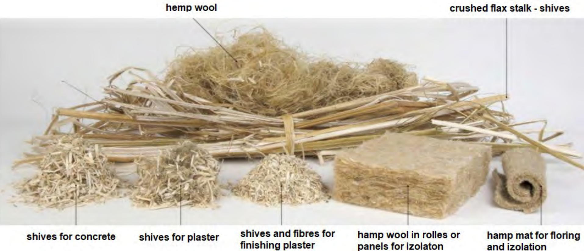
Fig. 3 Demonstration of semi-products in the processing of hemp fibers
