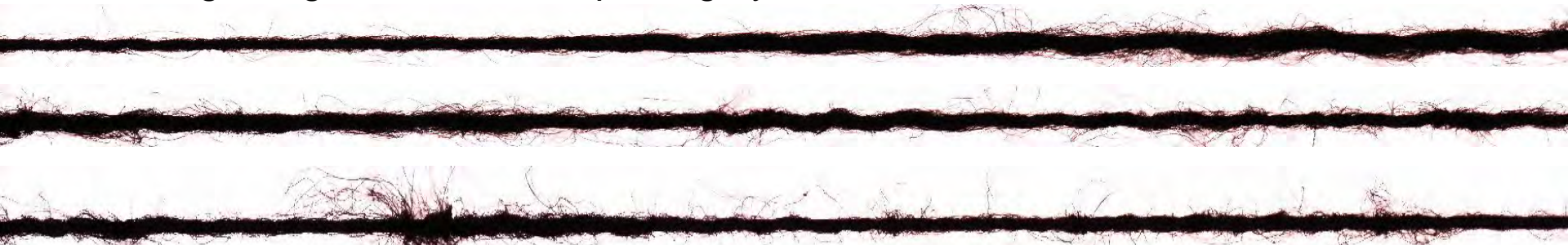
Fig. 24 An example of longitudinal views of yarns with piecing each 5 cm length
