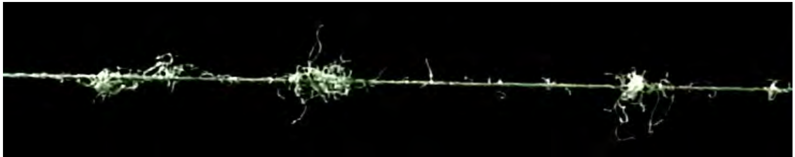
Fig. 30 100% CO 25 tex – after abrasion by applying 50 % of cycles need for yarn destruction (calibration 3,72\mu\text{m}\cdot\text{px}^{-1} , image resolution 548 pxl x 704 pxl)
