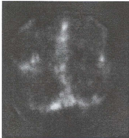
Figure 6.8 Typical irregular polygon-like convection pattern in the disordered medium at R = 1.27 . Reprinted from Howle (1993), with the permission of the author
