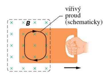
Aplication to electromagnetic brakes, induction heating etc.
