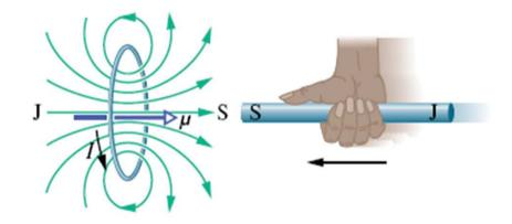
An induced emf is always in a direction that opposes the original change in flux that caused it.
