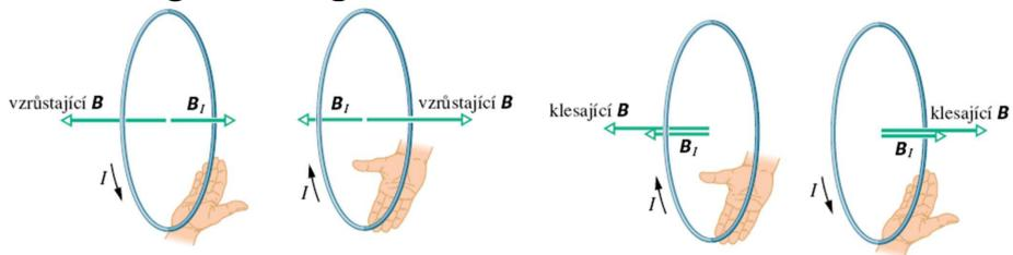
Current produced by an induced emf moves in a direction so that the magnetic field created by that current opposes the original change in flux.
