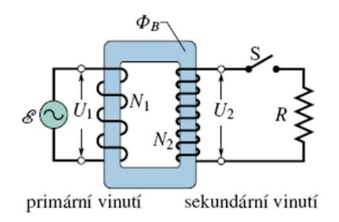
electromagnetic induction – common magnetic flux in transformer core
