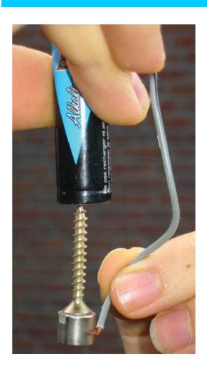
Movement due to the reaction of Lorentz's force on moving charge carriers
