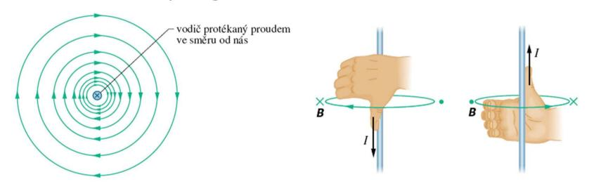
Wrap fingers around wire with thumb pointing in direction of current – fingers curl in direction of magnetic field.
