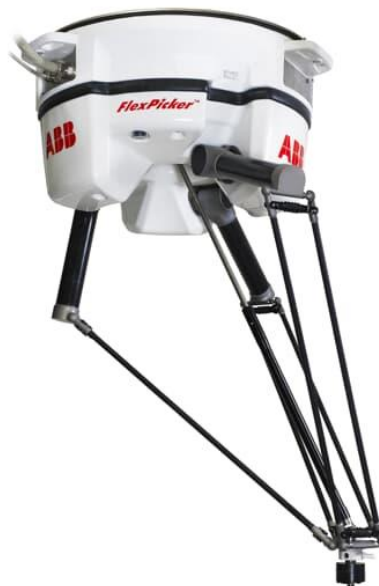
Delta-robot ABB FlexPicker IRB 360, foto: https://new.abb.com/
