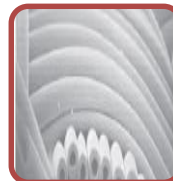
(f) nylon fibers with hollow cross-sections in a woven fabric
