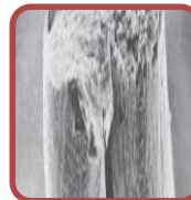
(h) acrylic fiber showing a dog-bone shaped cross-section.
