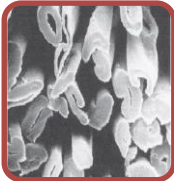
(b) view of cross-sections of cotton fibers showing their characteristic dog-bone shape
