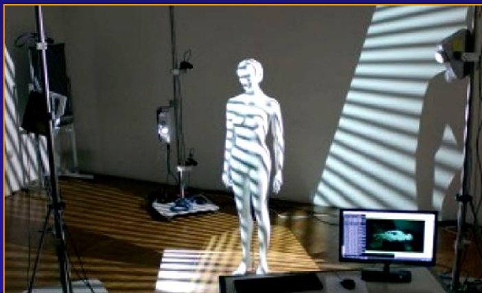
Princip structured light scannování [21]
