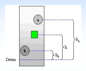
In this method the density of a material is determined by the density-gradient technique. A material is placed in a liquid column of variable density with standard floats (glass beads of known density). The material must float between a pair of the floats. The density of the material is then calculated based on its position in the column and the densities of the glass beads
