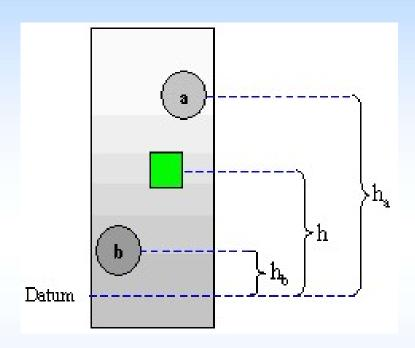
Density gradient column Graduated column with working length of 70cms
