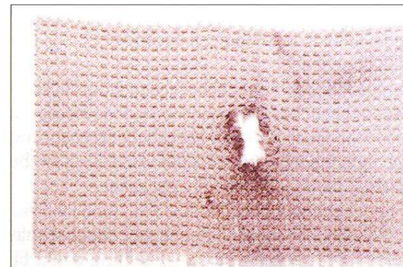
Fig. 82. Cotton fabrics with small holes after bleaching, typical of catalytic bleaching damage. Areas of damage with positive Oxycarmin test.
