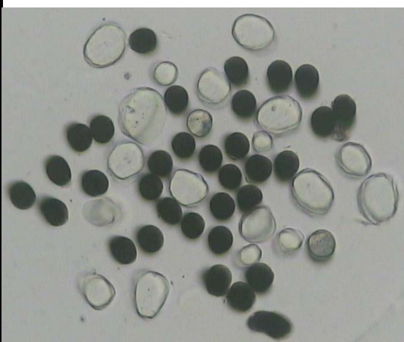
Cross section of ring spun yarn 20 tex, 65% PES/35% WO
