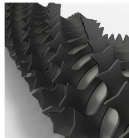
Detail of opening roll – Unifloc - fa Rieter
