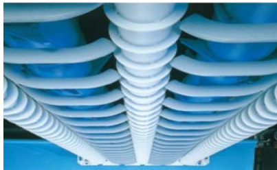
Production is distributed to two opening rolls. Three supporting rolls guarantee a solid stand of the bales.
