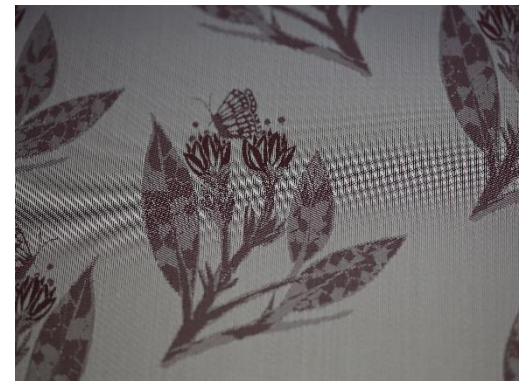
Structure of woven fabric given by jacquard shedding mechanism
