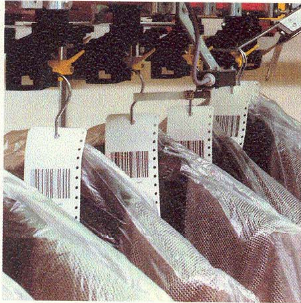
A scanner reads the data on the tag.
