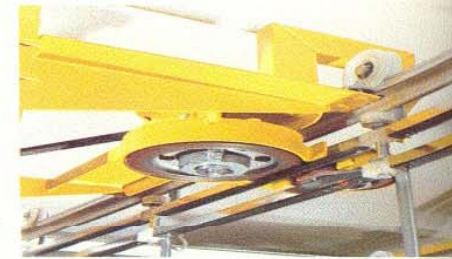
Low noise friction drive unit
