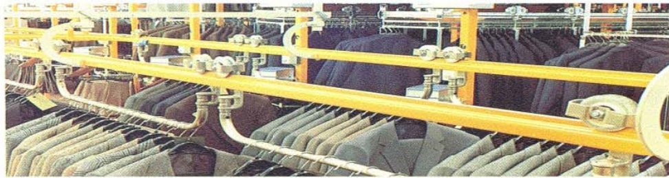
The material will be transported to the Wanderregal units by means of the DÜRKOPP overhead rail trolley system
