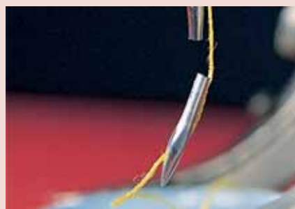
THE NEEDLE CAN BEND AND BREAK.
