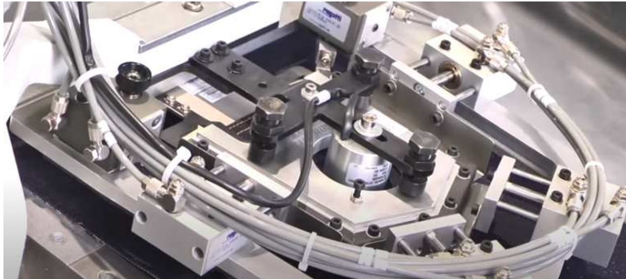
PFAFF 3588 Programmable automatic pocket setter
