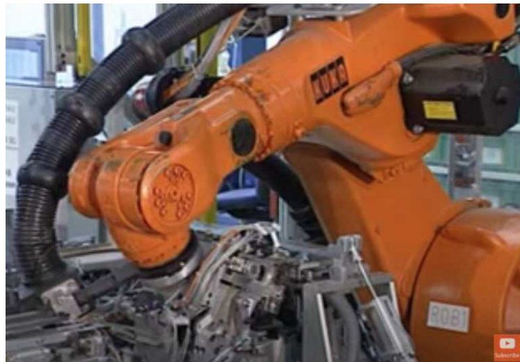
KUKA robot sews car seat covers
