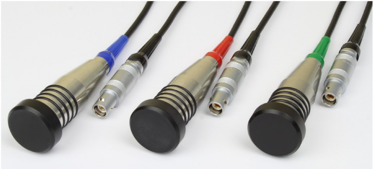
Fig. 10: Ultrasonic single-element transducers (blue: 1 MHz, red: 2 MHz, green: 4 MHz)
