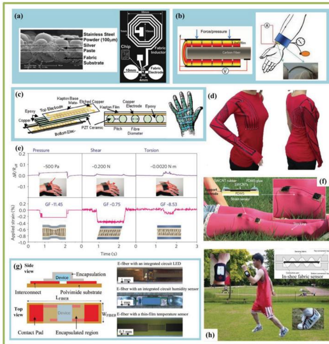
Figure 8. Fiber-based sensors: (a) Fabric bio-potential electrode and its SEM photo, Reproduced with permission. [144] Copyright 2010, IEEE. (b) Pulse-driven fiber nanogenerator by ZnO thin films grown around a carbon fiber as a strain sensor, Reproduced with permission. [6a] Copyright 2011, WILEY-VCH Verlag GmbH & Co. KGaA, Weinheim. (c) Vibration sensor arrays of piezoelectric fibers in gloves for detection and suppression of Parkinson's tremor in the hand, Reproduced with permission. [145] Copyright 2009, Textile Bioengineering and Informatics Society. (d) Carbon loaded elastomer sensorized garment for kinesthetic monitoring, Reproduced with permission. [146] Copyright 2011, Cambridge University Press. (e) Strain-gauge sensor based on the reversible interlocking of Pt-coated polymer nanofibres, Reproduced with permission. [140k] Copyright 2012, Nature Publishing Group. (f) Carbon nanotube strain sensor for human motion detection, Reproduced with permission. [20c] Copyright 2011, Nature Publishing Group. (g) Woven electronic fibers with sensing and display functions, Reproduced with permission. [5b] Copyright 2010, WILEY-VCH Verlag GmbH & Co. KGaA, Weinheim. (h) In-shoe plantar pressure monitoring in daily activities by fabric pressure sensors. Reproduced with permission. [140j] Copyright 2010, IEEE.
